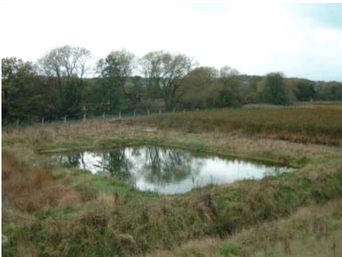
Figure 5.36.9. First cell of experimental wetland area from which plants have been removed to allow investigation of plants and algae in the ammonia removal process.
