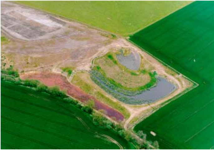
Figure 5.30.1. Aerial view of the Shilbottle constructed wetland and part of the spoil heap – the red-coloured area towards the left is the lower wetland cell which receives most of the spoil heap leachate (photo courtesy of Aln Elliot).
